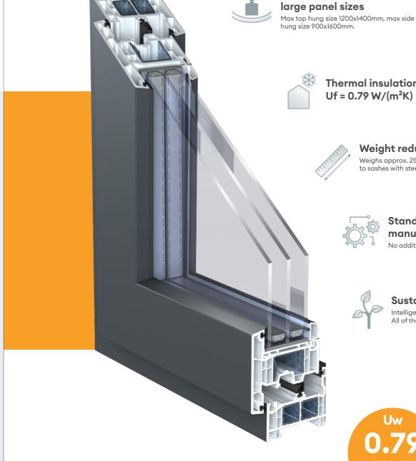
Thermal insulation value  $Uf = 0.79 W/(m^2K)$ Weight reduction Weighs approx. 25% less compared to sashes with steel. **Standardised** manufacture No additional steps required. Sustainability Intelligent recycling process.
